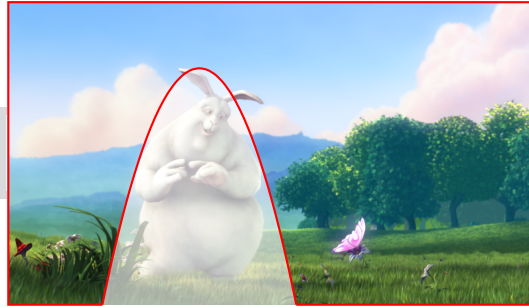
■ Figure 13 Two-dimensional segmentation of a screenshot from Big Buck Bunny [8] using a quadratic equation to define a cut. The URI must indicate which side of the cut to keep, either as a Boolean value or as an inequality. The URIs on the left yield the segment visualized on the right.
