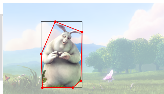
■ Figure 7 Polygonal segmentation of a 700 \times 400 screenshot from Big Buck Bunny [8]. The URIs of absolute and relative point coordinates on the left correspond to the visualization on the right. The polygon is shown in red, and the resulting image is outlined in black, where pixels outside of the polygon are turned transparent.
